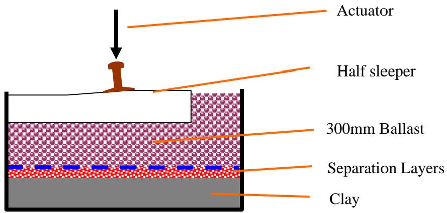
**a – section through box showing a typical test set-up**
